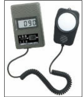
A light meter similar to the one used by Green Campus Interns to recommend de-lamping
