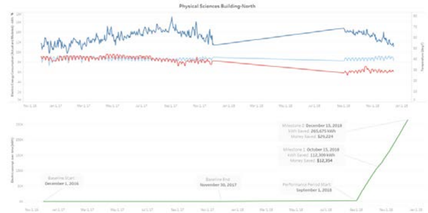
Preliminary electrical energy savings data for PSBN. Extrapolating first 2.5 months of savings to an annual sum gives $144k/yr in electrical energy savings, exceeding anticipated ROI.
